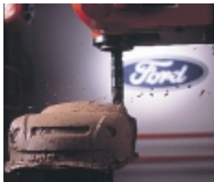
A computer-aided milling machine cutting a clay model.
